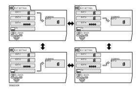
The arrow in the menu represents a signal flow. The left side of the arrow shows a signal source output from the EXT-2 terminal.
